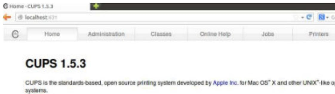
Click on the **Printers** tab to see a list of installed printers
